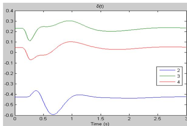
Figure 12: Rotor Angle Variation Δ after Optimization
