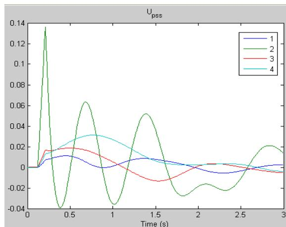
**Figure 7: Power System Stability Constant  $U_{PSS}$  before Optimization**
