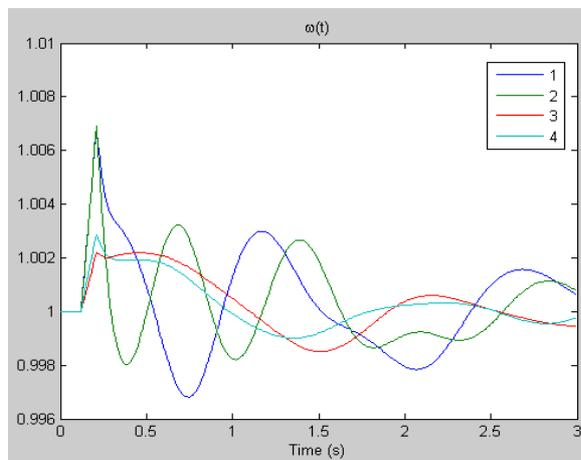
**Figure 9: Rotor Speed Variation  $\omega$  before Optimization**
