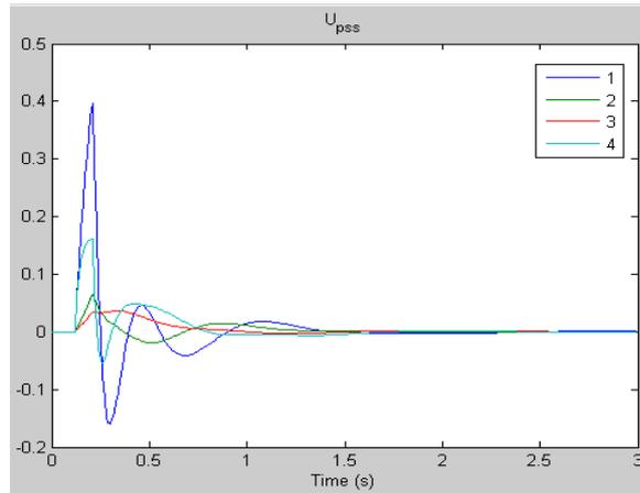
**Figure 8: Power System Stability Constant  $U_{PSS}$  after Optimization**
