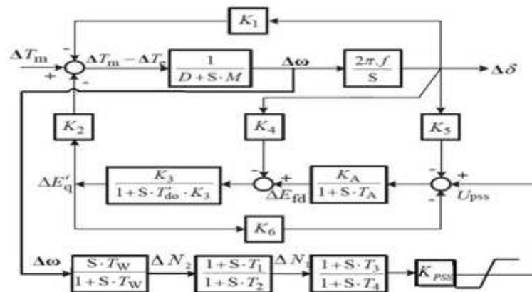
Figure 4: Linearized Model of SMIB System with PSS Attendance
