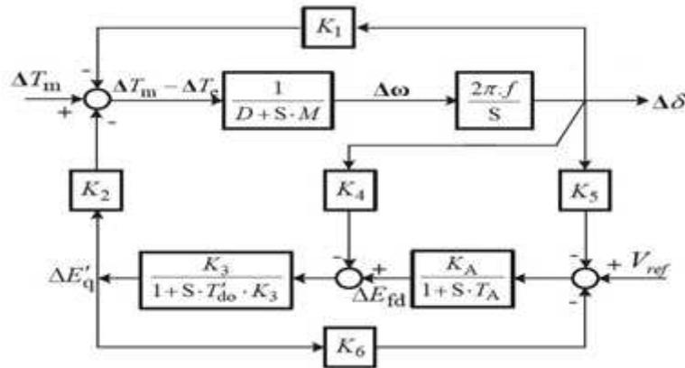
Figure 3: Linearized Model of SMIB System
