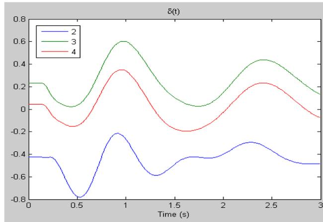
Figure 11: Rotor Angle Variation Δ before Optimization
